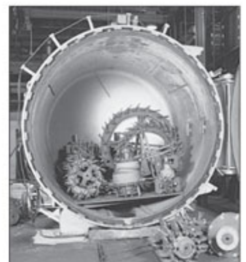
A range of products in the open autoclave before closing the door and steam curing for approximately 3 hours at 305° F (151°C).
