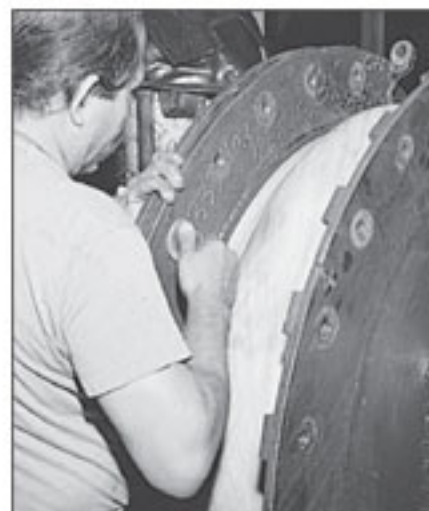
Forming the rubber flanges with steel flange rings after the Nylon tape has been wrapped over the expansion joint body to hold the shape during the curing process. Flanges must be built correctly to maintain seals and avoid pullout.
