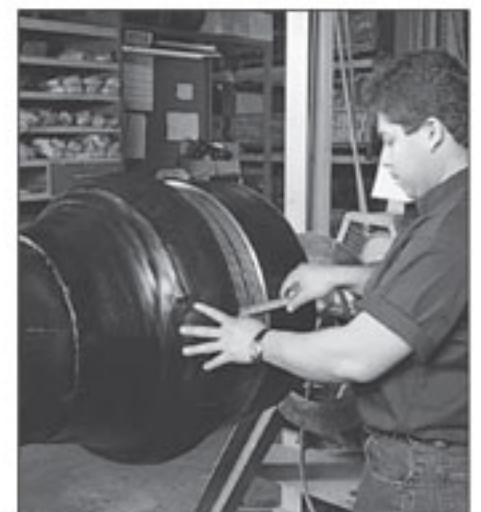
Checking steel wire reinforcement spacing. This guarantees consistently high safety factors.
